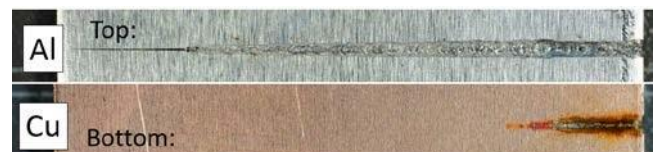
Fig. 9 1.5 mm Al welded on 0.4 mm Cu with increasing power, the same sample is shown from top and bottom side.
